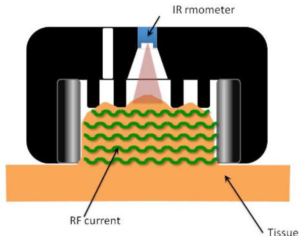
**Figure 1 - Hand piece geometry demonstrating RF current passing through the tissue in the suction cavity**
